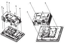
3. Remove the communication card, if necessary, to access the battery.
