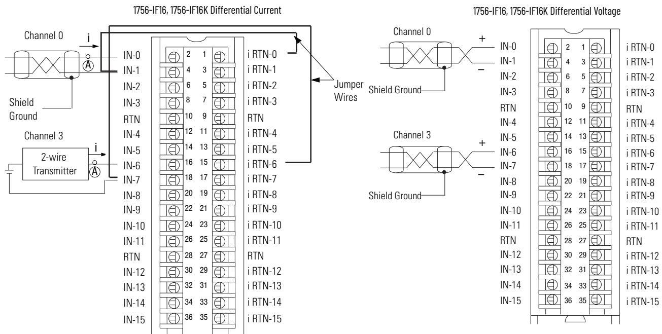
Use this table when wiring your module in Differential Current mode.
